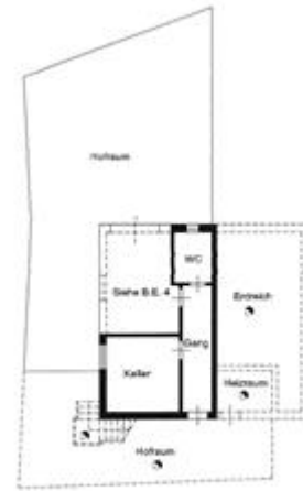
ERDGESCHOSS H = 2,40 m
